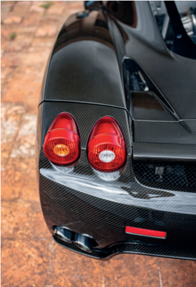
It's harder than it looks: bare and unpainted, carbon fibre doesn't tolerate any imperfections in its weave.
