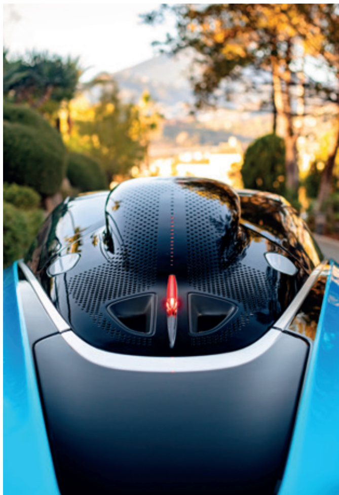
The engine's dual air intakes, separated by the third vertical brake light, are built into the roof so as not to disrupt the flow of air around the body.
